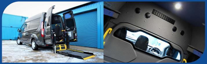
The council requested that the vehicle included a custom-built bulkhead with a protective screen. The screen enables them to provide these essential services without putting their clients or drivers at risk. The rear saloon also features a completely separate heating and air conditioning system allowing both driver and passenger to remain comfortable without the worry of recirculating air.
