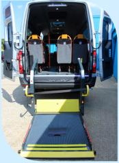
Inside, we have finished the minibuses in a colourful orange and red design with twin belted passenger seats that feature a state-of-the-art 'All Buckled Up' system. The 'All Buckled Up' system uses wireless technology to audibly and visually inform the driver of passenger seats with unbuckled seatbelts.
