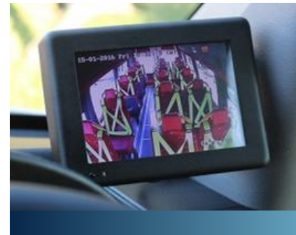
INTERNAL CCTV MONITOR
