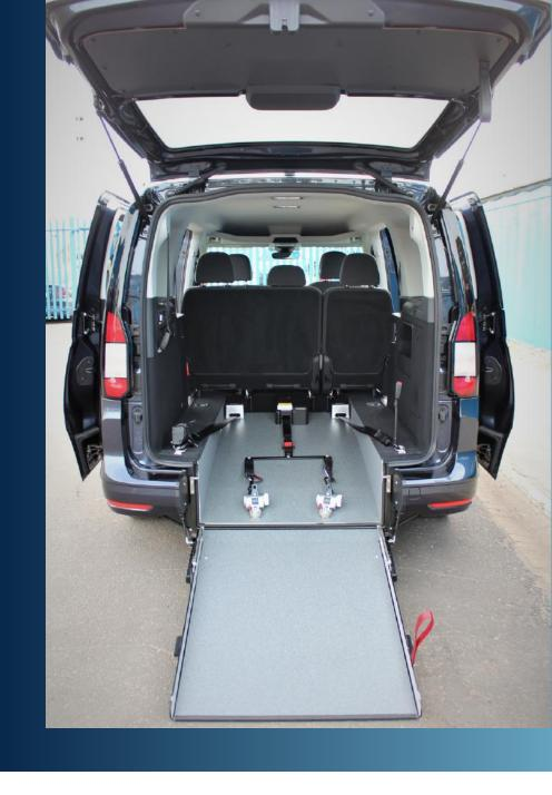
Specially designed cut-in floor for wheelchair passengers.
