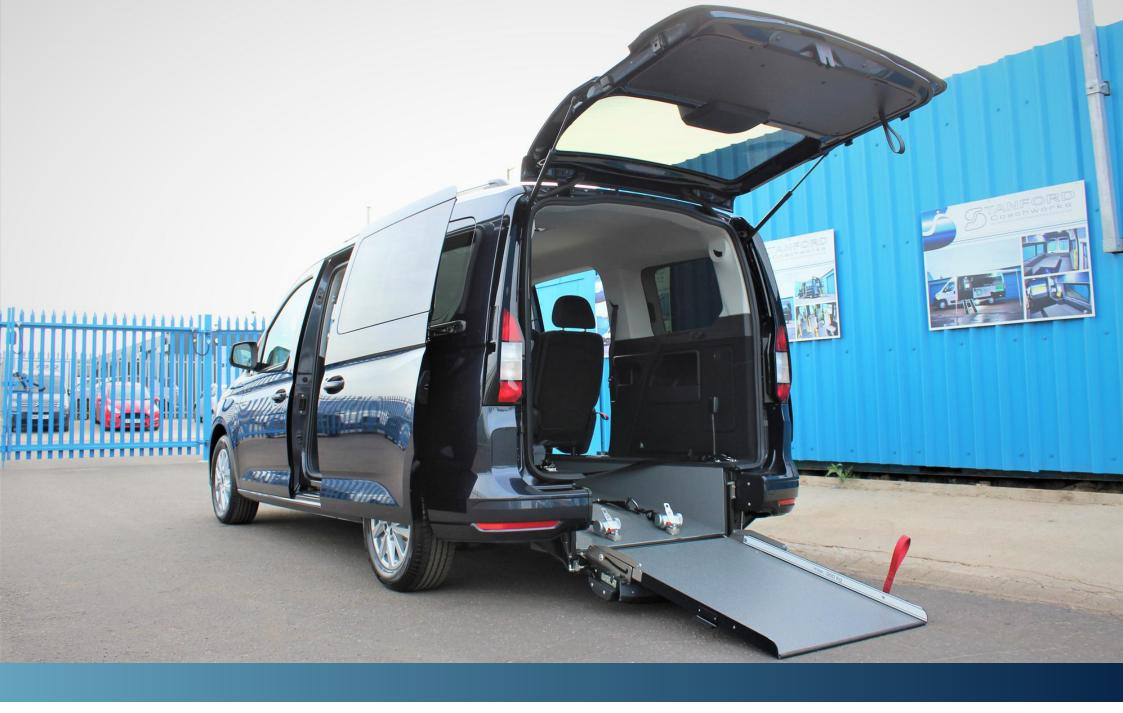
Specially designed fold-out ramp which sits inside of original vehicle flooring.
