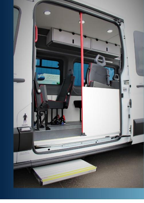
Passenger entry - heavy-duty ramp & electric side step
