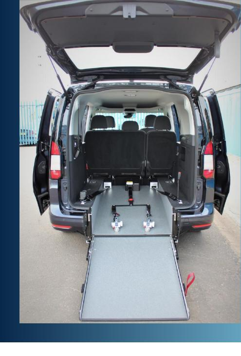
Passenger seating & specially designed cut-in floor
