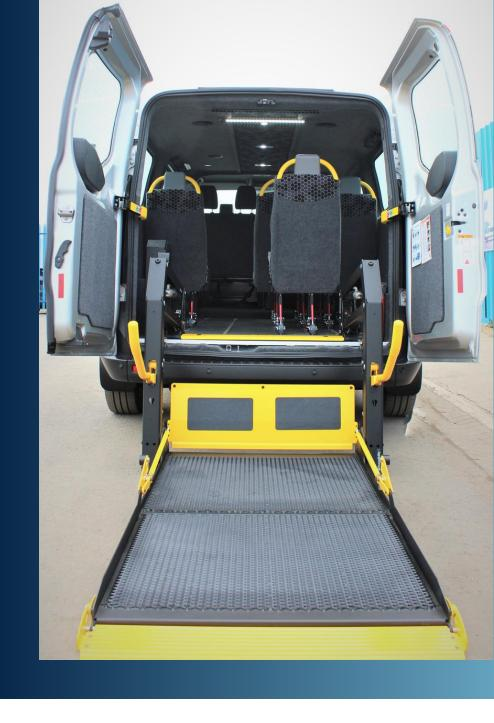
Passenger entry - pedal operated side step & internal tail lift
