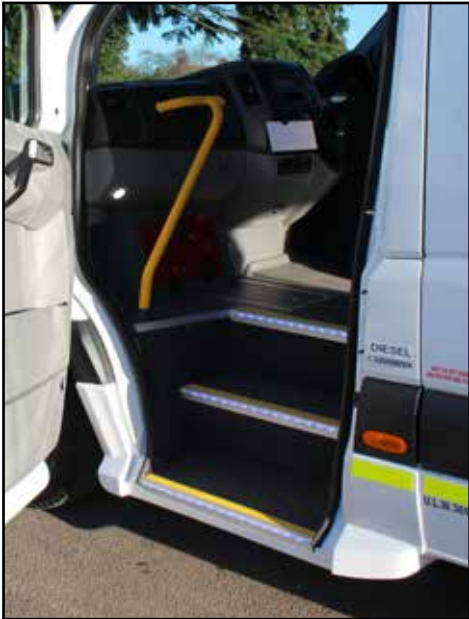
Cut in front entry Available on: Iveco Daily, Mercedes Sprinter, Volkswagen Crafter
