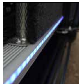
LED entry lighting strips
